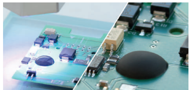
Defined glob top encapsulation within seconds (left during curing, right after curing)
