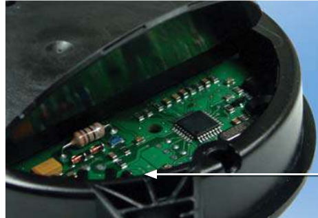
Fixing / sealing of a PCB in a housing (© viaSonic)
