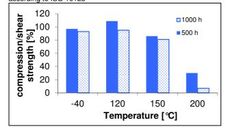
compression/shear strength shaft-hub joint at temperature based on initial valve at room temperature measured at determined temperature
