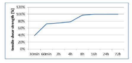
compression shear strength shaft-hub joint with activator DELO-QUICK 5006 based on initial value at room temperature measured at room temperature (approx. 23 ℃) according to ISO 10123
