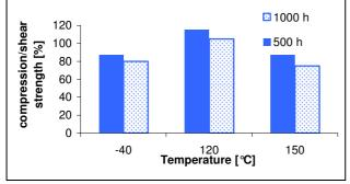
tensile strength after temperature storage based on initial value at room temperature measured at room temperature (approx. 23 °C)
