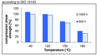
compression/shear strength shaft-hub joint at temperature based on initial value at room temperature measured at determined temperature according to ISO 10123
