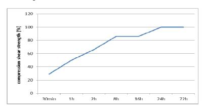
compression shear strength shaft-hub joint with activator DELO-QUICK 5006 based on initial value at room temperature measured at room temperature (approx. 23 ℃) according to ISO 10123
