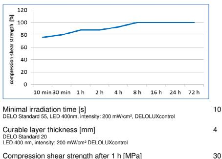
Compression shear strength [MPa] according to ISO 10123 Compression shear strength glass/glass [MPa] DELO Standard 5 LED 400 nm, intensity: 200 mW/cm<sup>2</sup> DELOLUXcontrol, irradiation time: 60 s Tensile shear strength AI/AI [MPa] DIN EN 1465
