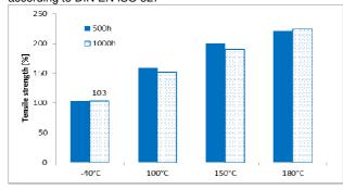
elongation at tear after temperature storage based on initial value at room temperature measured at room temperature (approx. 23 °C) according to DIN EN ISO 527
