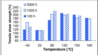
based on initial value at room temperature measured at determined temperature according to DIN EN 1465
