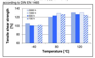
Tensile shear strength Al/Al sand- blasted at temperature related to the initial value at room temperature measured at temperature according to DIN EN 1465
