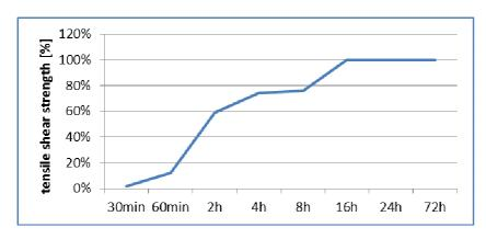
compression shear strength shaft-hub joint with activator DELO-QUICK 5006 based on initial value at room temperature measured at room temperature (approx. 23 °C) according to ISO 10123
