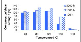
compression/shear strength glass/glass at temperature based on initial value at room temperature measured at determined temperature according to DELO standard 5
