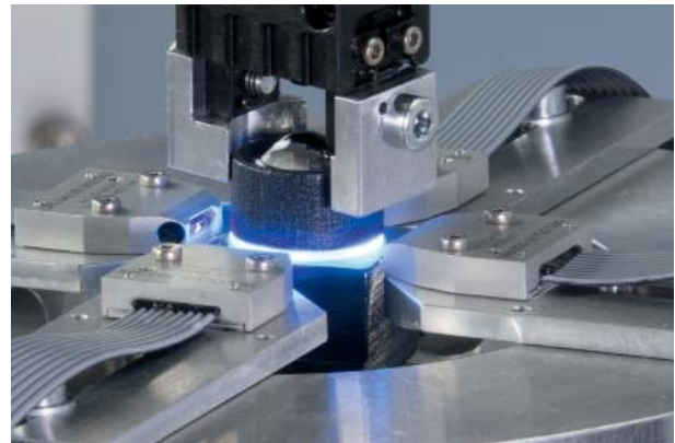
Adhesive curing in compact camera modules using 4 DELOLUX 502 heads
