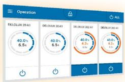
**Process control:** Irradiation parameters of up to 4 lamp heads are displayed simultaneously in the main menu and controlled via touch screen. Several user languages make the device ideally suited for international use.
