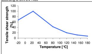
tensile strength after temperature storage based on initial valve at room temperature measured at room temperature (approx. 23 °C)
