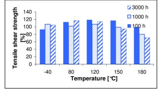
based on initial value at room temperature measured at determined temperature according to DIN EN 1465
