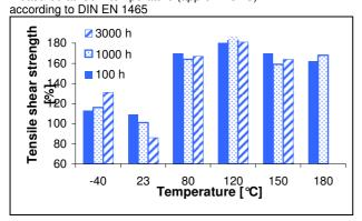
tensile shear strength Al/Al sand- blasted at temperature based on initial value at room temperature measured at determined temperature according to DIN EN 1465
