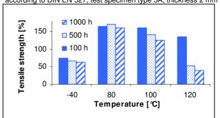
elongation at tear after temperature storage based on initial valve at room temperature measured at room temperature (approx. 23 °C)
