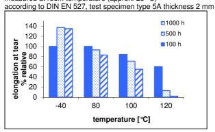
tensile strength after temperature storage based on initial value at room temperature measured at room temperature (approx. 23 °C)
